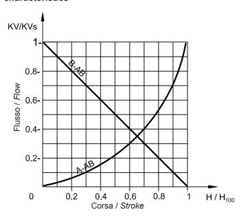
A-AB equal-percentage way B-AB bypass lineare way 3-way used as mixing inlet in A and B, outlet AB 3-way used as diverting inlet in AB, outlet from A and B
