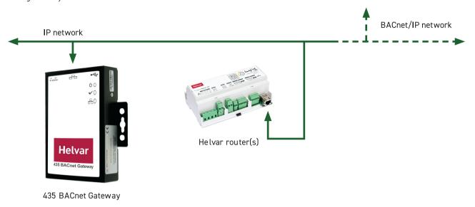
The BACnet Gateway allows a BMS to control and monitor the lighting system as well as obtain device status and group power consumption information. BACnet/IP clients can easily connect with the gateway via a TCP/IP network.
