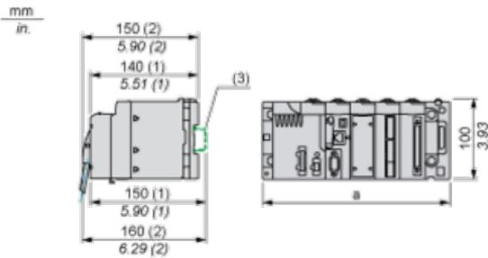
(1) With removable terminal block (cage, screw or spring).
