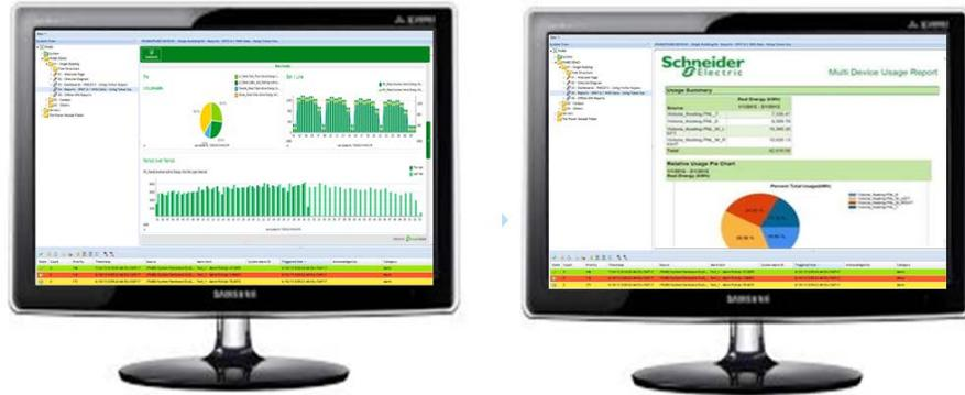
The PME Dashboards and Reports applications utilize logged trend data only from the PME database. Therefore, any data from SBO that is to be displayed in a Dashboard or Report needs to be in the PME database.
