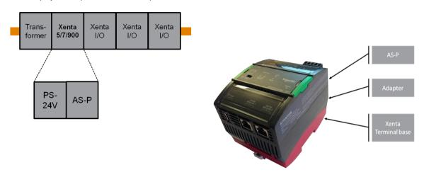
To avoid the need for rebuilds, the Xenta to AS-P Adapter allows the AS-P and Power Supply to be inserted conveniently into the space where Xenta 500/700/911/913 was mounted. The Xenta terminal base stays and thus no re-wiring is required. The adapter includes the power supply for the AS-P.
